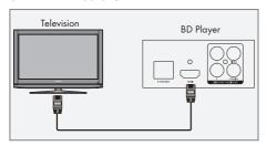
1 Connect an HDMI cable (not supplied) into the »HDMI« socket on the back of the device and the corresponding socket (HDMI) on the LED/LCD TV.
